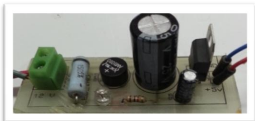
Fig 3 power supply board
