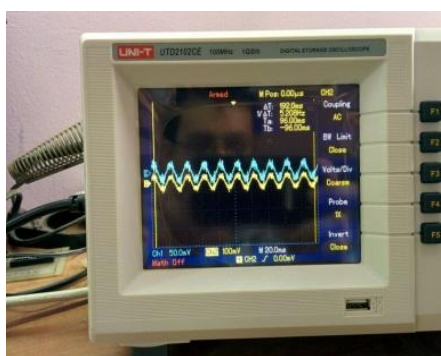
Fig 8 oscilloscope signal after improving PF
